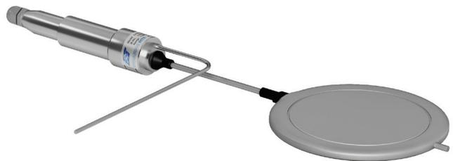
For applications in which the concrete pressure cell is embedded in concrete, a 600 mm long, fluid filled, pinch tube is welded to the sensor.
