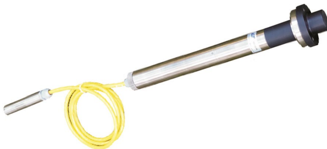
Figure 2 Datalogger with sensor
