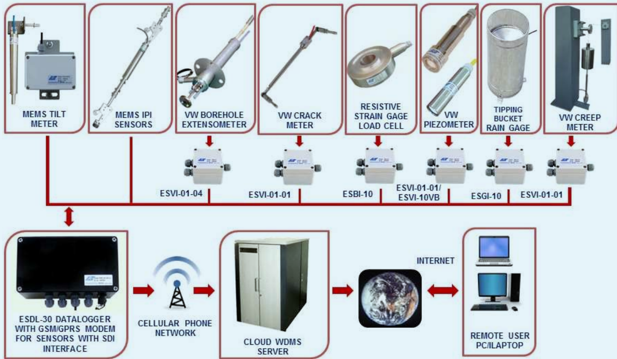
Fig. 3 : Different Sensors Connected through SDI-12 Bus Cable to a Data Logger with Web Based Data Monitoring
