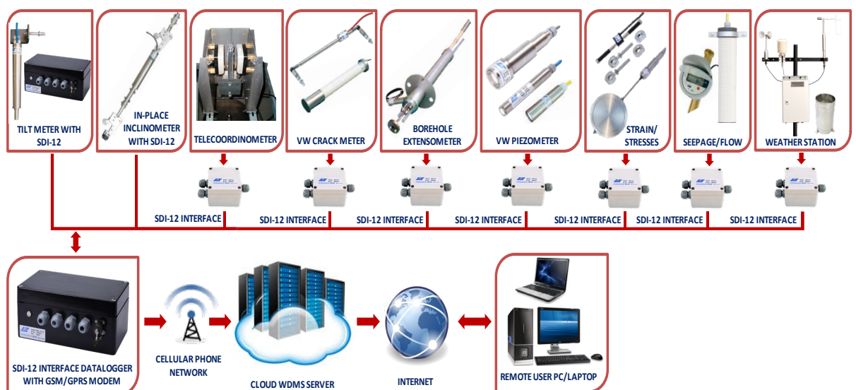
Fig. 5 Dam monitoring instruments on an SDI-12 network
