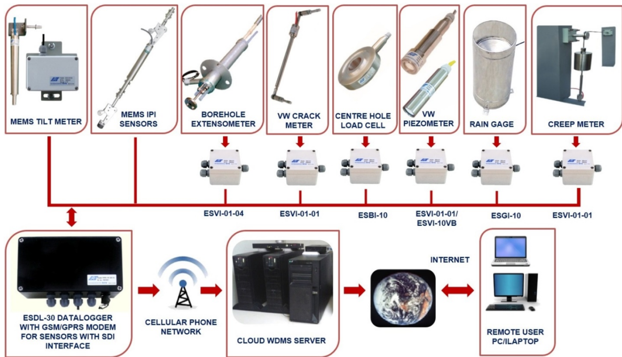
Figure 5: Slope stability sensors on a SDI-12 network
