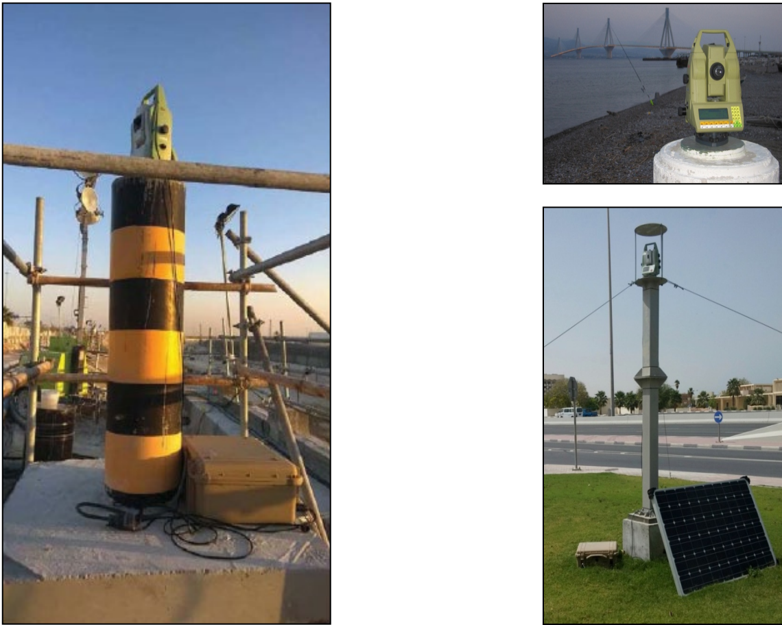
Figure 3: ATS with different mounting arrangements
