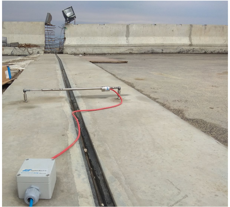
Displacement sensors installed to measure free and fixed bearing movement and expansion joints
