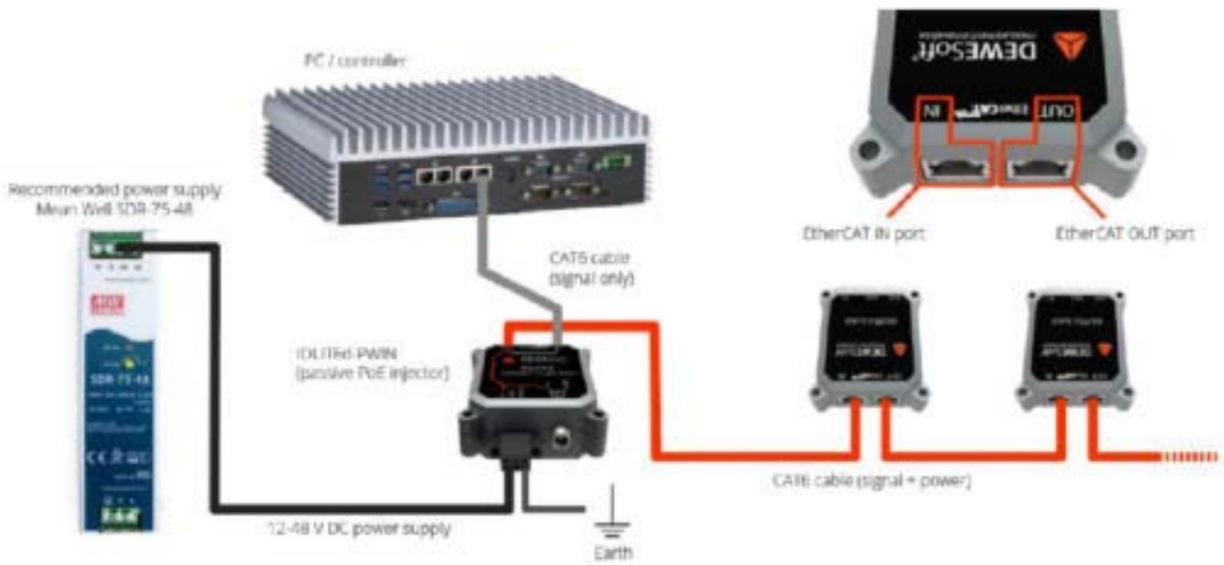
EtherCAT based accelerometer network
