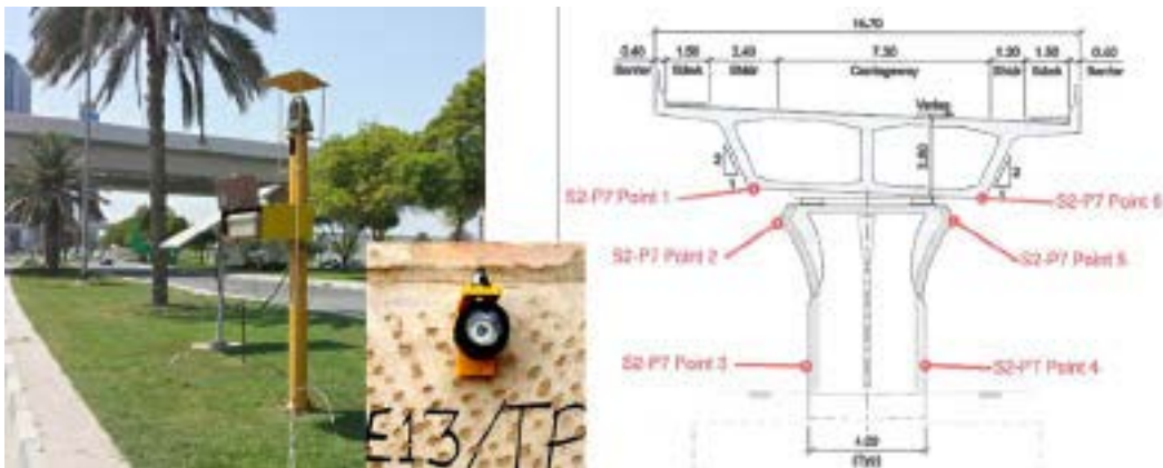
Web-based monitoring of lateral movement and settlement using robotic total stations and prism targets
