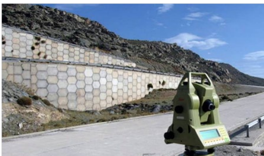
Automatic surveying system (ATS)
