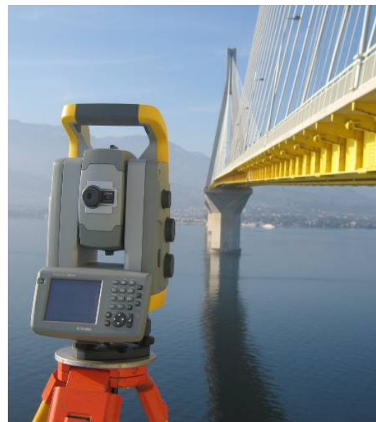
Structural monitoring using ATS
