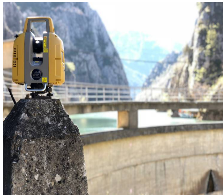
Automatic surveying system (ATS)
